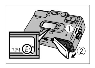
When the exposure counter shows "  $\xi$  " and the motor stops, move the film cartridge compartment cover release knob as indicated in ①, in the direction indicated in ②, and open the film cartridge compartment cover.
